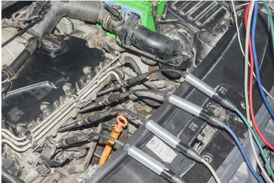
Fig 11. Measuring pressure in cylinders with BERU glow plugs and signal amplifiers
